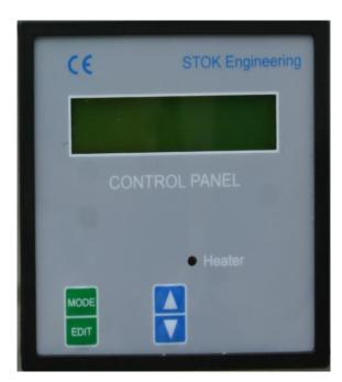
Setting the operating temperature: Press the MODE button once. Press the EDIT button three times until TEMPERATURE = 190 appears on the display. With  $\triangle$  and  $\nabla$  buttons you can change the factory preset temperature. (The default setting is 190° C). Press the MODE button once again and the machine is ready to run.
